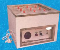
Water Bath Rectangular (Double Wall): Outer body made of mild steel painted with white stoving enamel. Inner chamber made of thick S/Steel complete with concentric rings. Temperature controlled by hydraulic thermostat from ambient to 95°C, +/- 1°C. Complete with control panel but without Thermometer. To work on 220/230 VAC.
